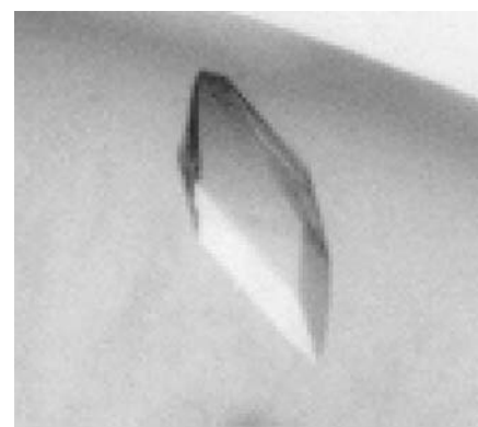
Figure 3 Crystal of A. aeolicus dihydroorotase. An A. aeolicus DHOase crystal, 0.2 mm in the longest dimension, was obtained by the hanging-drop method at 295 K using 1 M lithium sulfate, 100 mM Tris acetate pH 8.5 and 10 mM nickel chloride hexahydrate in the well. The protein (6.7 mg ml -1 , 0.002 ml) in 50 mM HEPES pH 7.4 was diluted 1:2 with the precipitating solution. The crystal was grown for ten weeks.
